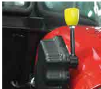
60X, 70X, 80X Models External Hydraulic Control
