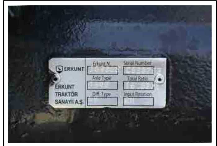
Erkunt front axle number is located on the left side of the front axle.
