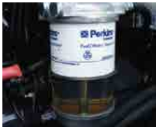
Water retaining filter
